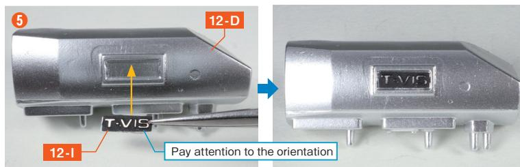
Cut one of the two pieces of **Double-Sided Tape 12-J**, peel off one backing sheet, and apply it to the back of the **T-VIS Plate 12-I**.
